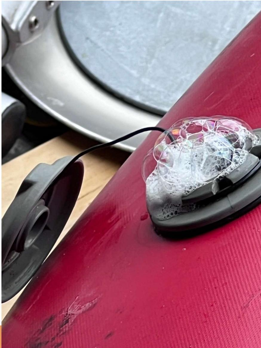
Spray the valve with soapy water, if the valve still produces bubbles after tightening and cleaning, it is time to replace the valve, the spring is broke or there is a crack letting air get out.
